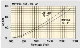
Bypass valve pressure drop
