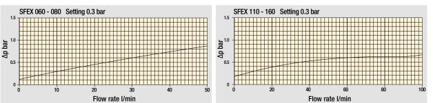
The curves are plotted using mineral oil with density of  $0.86 \text{ kg/dm}^3$  in compliance with ISO 3968.  $\Delta p$  varies proportionally with density.
